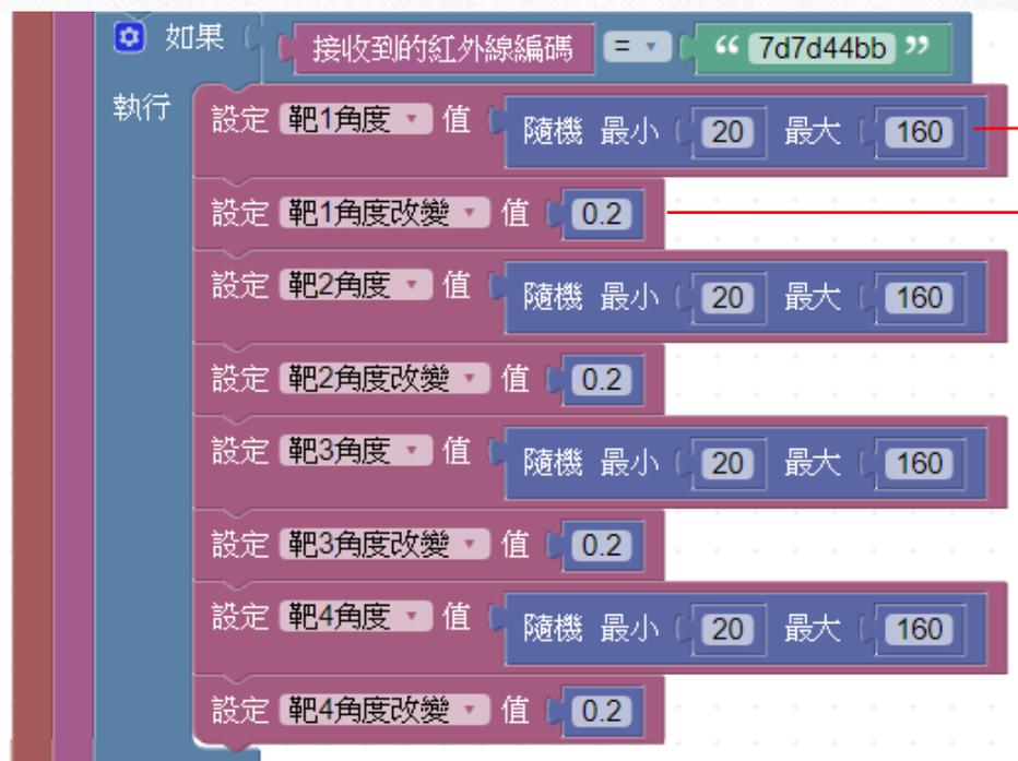
The image shows a Scratch script starting with an 'If' block that checks if the received infrared code is '7d7d44bb'. Inside the 'If' block, there are eight 'Set' blocks arranged in pairs for four targets. Each pair consists of a 'Set Target Angle' block and a 'Set Target Angle Change' block. The 'Set Target Angle' blocks are set to 'Random' with a minimum of 20 and a maximum of 160. The 'Set Target Angle Change' blocks are set to 0.2.
